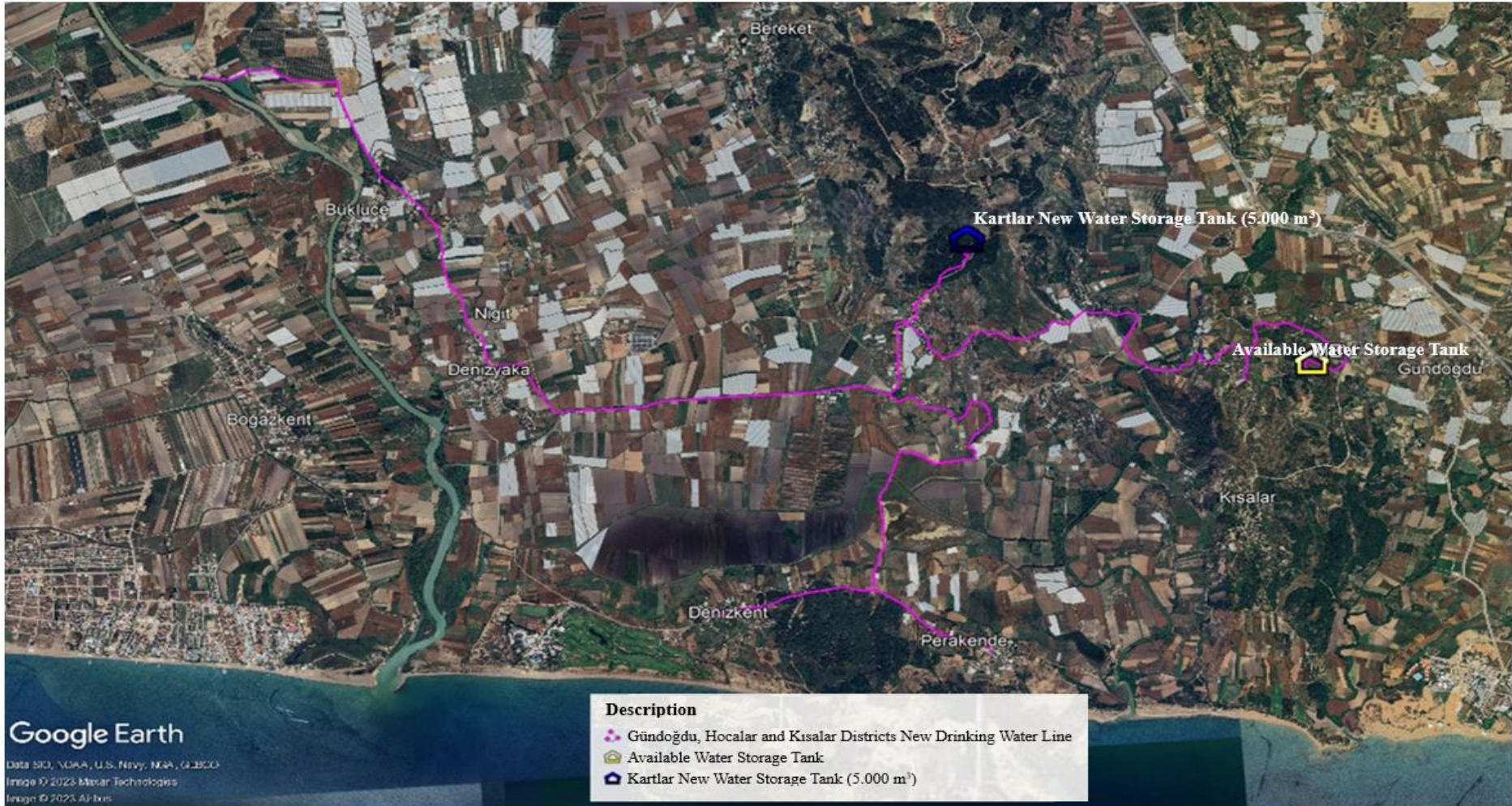
Figure 10: Drinking Water Storage Tank and Network Line in Districts affected by Wildfire (Manavgat; Gündoğdu, Hocalar, Kısalar Districts)
